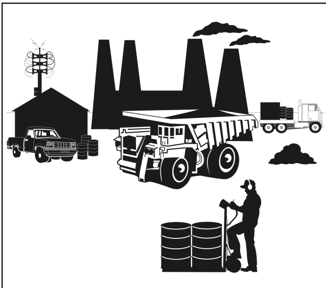
Figure 3. Unacceptable solution: Obstructions and noise producing machinery restrict intelligibility of alarm messages.
